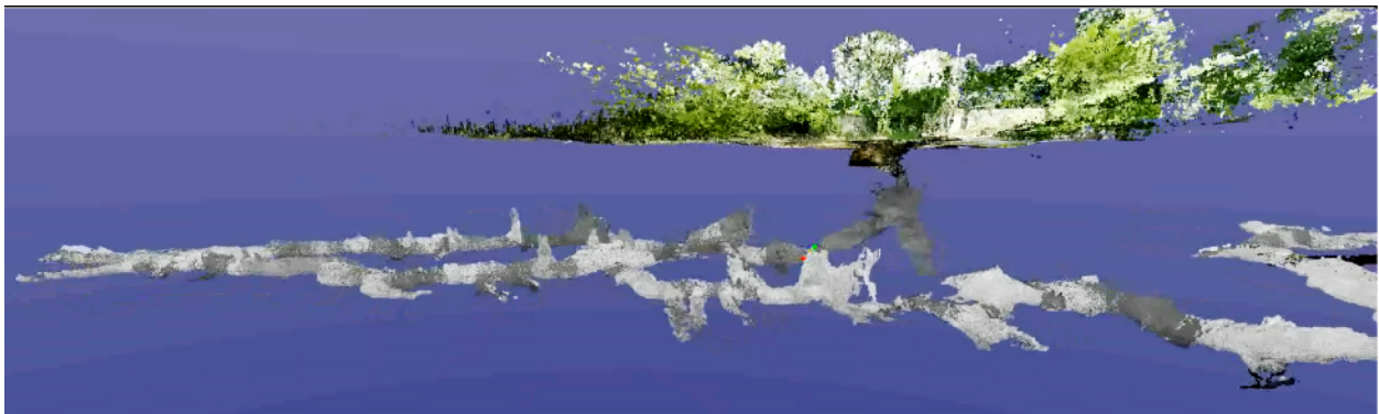
Images showing the result of the profile scan with the unevenness from the surface to the interior of the cave. The red dots correspond to the scanner stations
