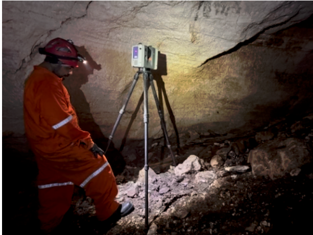
Documentation process with the Leica RTC360 scanner
